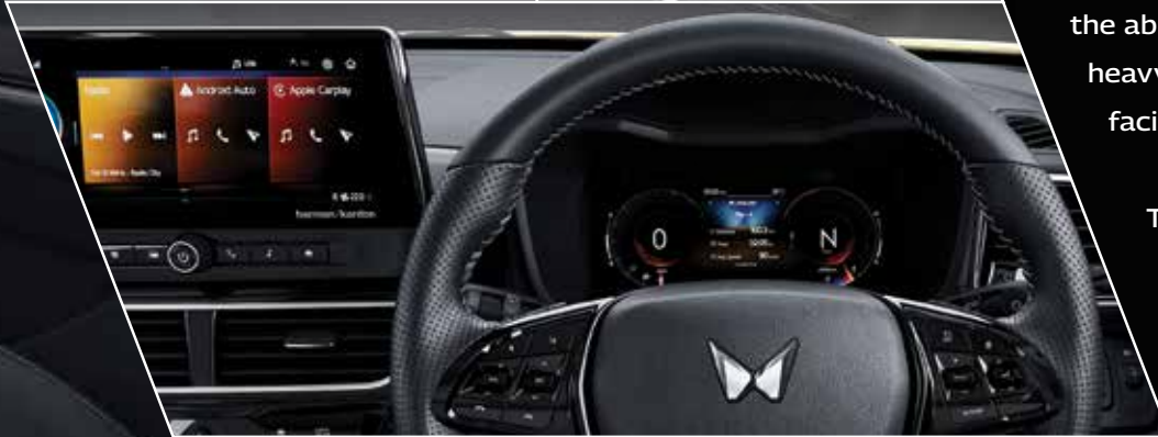
Dual floating high-resolution screens - with the largest 10.25" digital cluster and 10.25" infotainment system
